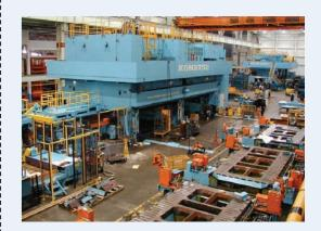
**IDDER** In response to needs in the U.S. auto manufacturing market, Komatsu develops fully-automatic transfer presses that deliver high-productivity features, such as fully automated die change and the first servo-controlled transfer feeder.
